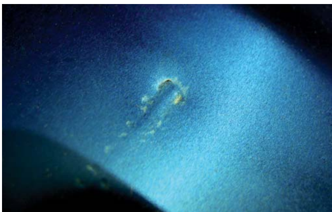
Figure 15: Mild damage of the absorber at the beginning of one of the welded seams.
