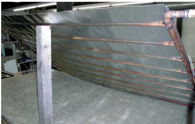
Figure 13: Backside of absorber following 1000th cycle.
