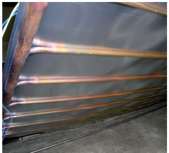
Figure 12: Backside of the absorber. All welded seams remain intact.
