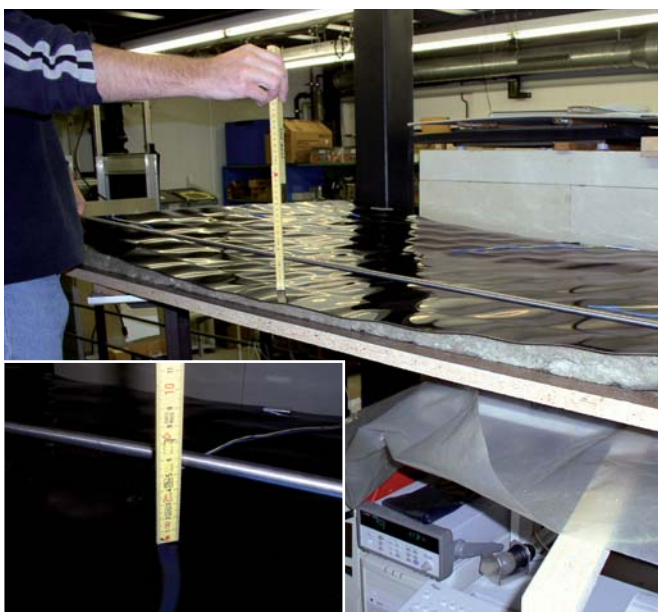
Figures 10 & 11: Significant dished deformation led to an overall curvature with a depth in the range of 5 - 6 cm.
