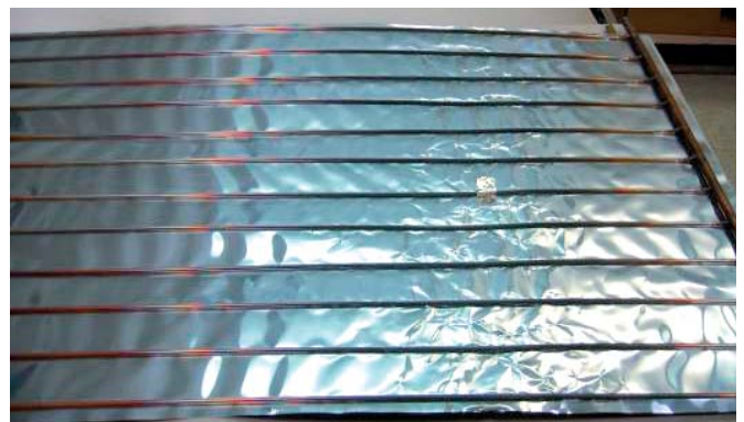
Images 1 and 2: Photo of the absorber after the shock test. Formation of ripples on the absorber plate.
