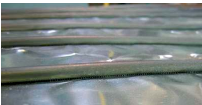
Images 3 and 4: Close-up photos showing the ripples on the absorber plate.
